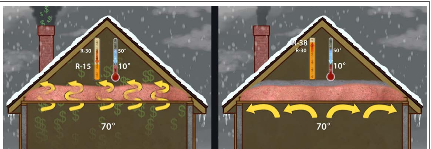
The 28 minute video utilizes computer animation to demonstrate how 50% of the “R” value with common blown-in fiberglass is lost as the attic temperature falls to 10°. The solution, according to scientists at Oak Ridge Laboratories, is to install a few inches of high density (1.6# PCF) cellulose insulation over the top of the low density fiberglass (.6# PCF).
