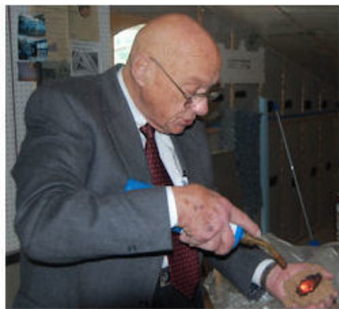
Richard Munson uses a blowtorch to demonstrate the insulating and flame retardant properties of his Celluborate fiber, made from 90 percent recycled cardboard. (J.W. Oliver photo)
